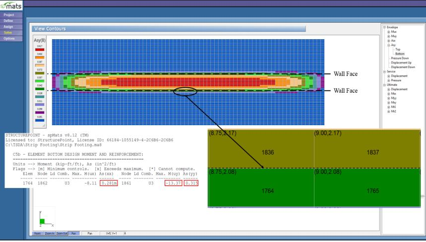
Figure 7 – Required Reinforcement Contour (spMats)
