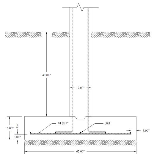
Figure 4 – Wall Footing Reinforcement Details
