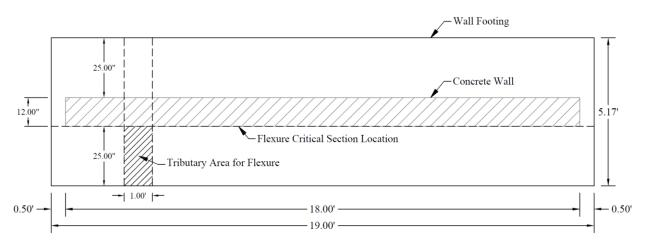
Figure 3 – Strip Footing Plan Showing Tributary Area for Flexure
