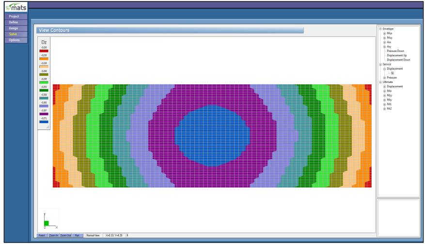
Figure 8 – Vertical Displacement Contour (spMats)
