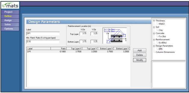
Figure 9 – Defining Design Parameters (spMats)
