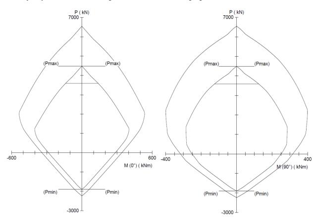
Interaction Diagram About the x-axis Interaction Diagram About the y-axis Figure 11 – Comparison of Column Interaction Diagrams about X-Axis and Y-Axis (spColumn)
