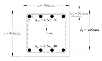
Figure 1 - Reinforced Concrete Column Cross-Section
