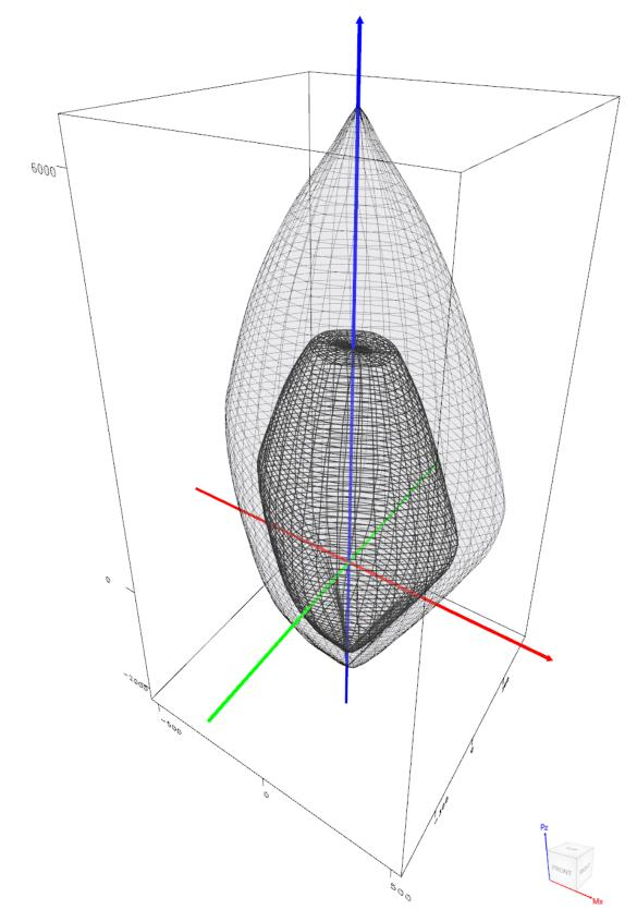
Figure 12 – Nominal & Design Interaction Diagram in Two Directions (Biaxial) (spColumn)
