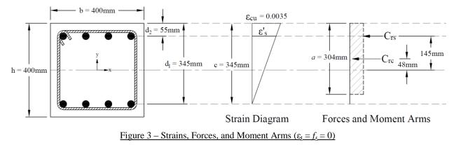
Strain  $\varepsilon_s$  is zero in the extreme layer of tension steel. This case is considered when calculating an interaction diagram because it marks the change from compression lap splices being allowed on all longitudinal bars, to the more severe requirement of tensile lap splices. <u>CSA A23.3-94 (12.15 and 16)</u>
