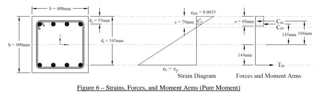
This corresponds to the case where the factored axial load resistance,  $P_r$ , is equal to zero. Iterative procedure is used to determine the factored moment resistance as follows:
