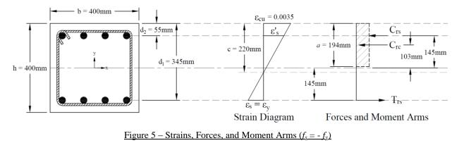
This strain distribution is called the balanced failure case and the compression-controlled strain limit. It marks the change from compression failures originating by crushing of the compression surface of the section, to tension failures initiated by yield of longitudinal reinforcement.
