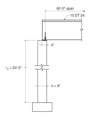
Figure 1 – Reinforced Concrete Precast Wall Panel Geometry
