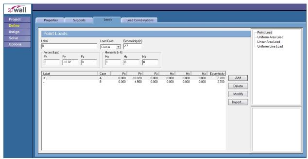
Figure 3 – Defining Loads for Precast Wall Panel (spWall)
