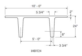
Eccentricity of the roof loads about the panel center line =  $\frac{2}{3} \times 4 = 2.7$  in.
