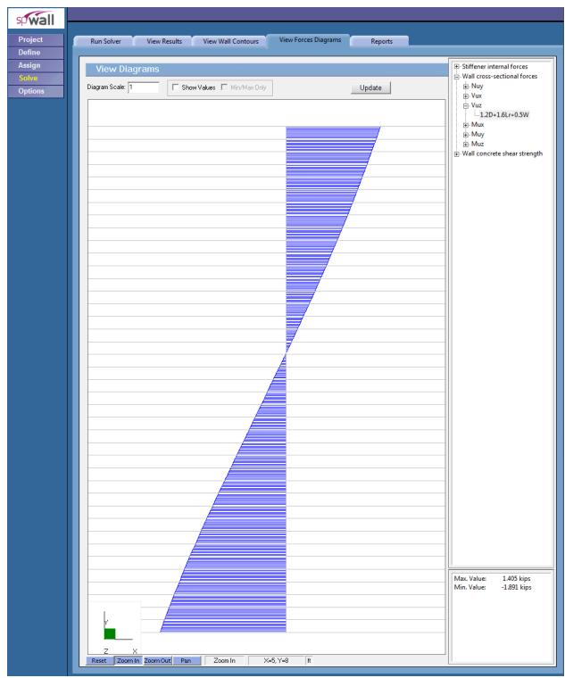
Figure 8 – Out-of-plane Shear Diagram (spWall)
