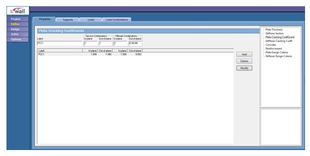
Figure 13 – Defining Cracking Coefficient (spWall)
