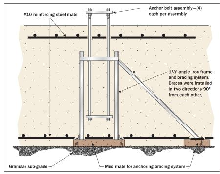
Fig. 1. Anchor Bolt Assembly Anchoring System. The anchor bolts were secured to "mud mats" placed in the subgrade. Angle irons placed at angles and secured to mud mats fixed the anchor bolts in proper position.
