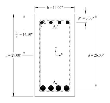
Figure 1 - Doubly Reinforced Concrete Beam Cross-Section
