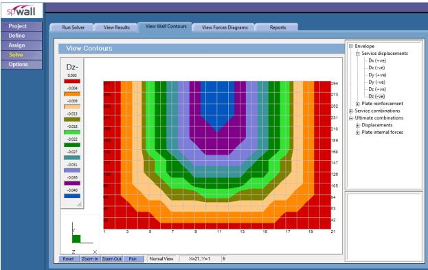
Figure 8 – Lateral Displacement Contour (Out-of-Plane)
