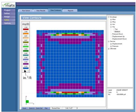
Figure 26 – Required Reinforcement Contour along Y Direction (Bottom)
