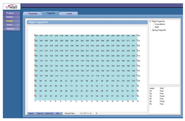
Figure 6 – Assigning Vertical Wall Restraints
