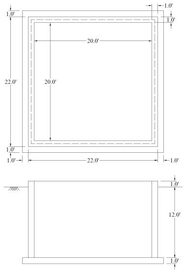
Figure 1 – Rectangular Concrete Tank Plan and Elevation
