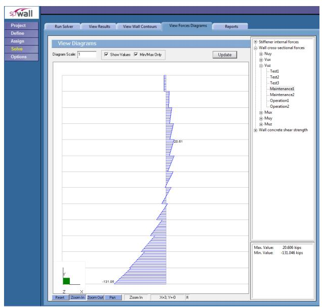
Figure 10 – Tank Wall Out-of-Plane Shear Diagram
