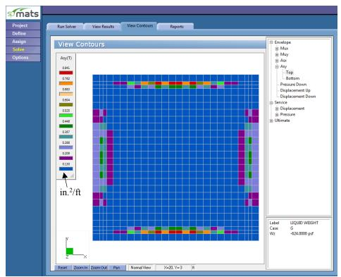
Figure 27 – Required Reinforcement Contour along Y Direction (Top)
