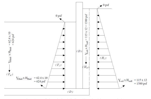
Figure 2 – Applied Loads (1 and d indicated lateral and down respectively)
