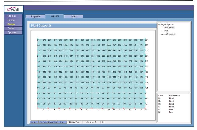
Figure 5 – Assigning Horizontal Wall Restraints
