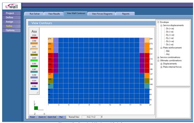
Figure 17 – Required Horizontal Reinforcement
