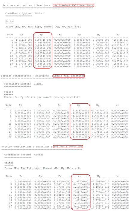
Figure 15 – Wall Reactions (Service Combinations)
