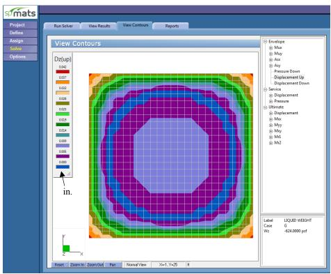
Figure 22 – Vertical (Up) Displacement Contour
