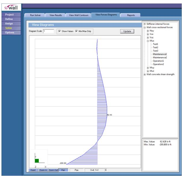
Figure 11 – Tank Wall Bending Moment Diagram
