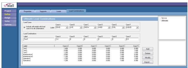
Figure 3 –Defining Tank Wall Loads and Load Combinations
