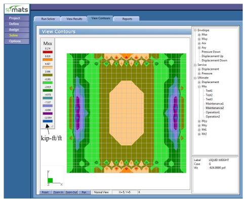
Figure 25 – Moment Contour along X-Axis
