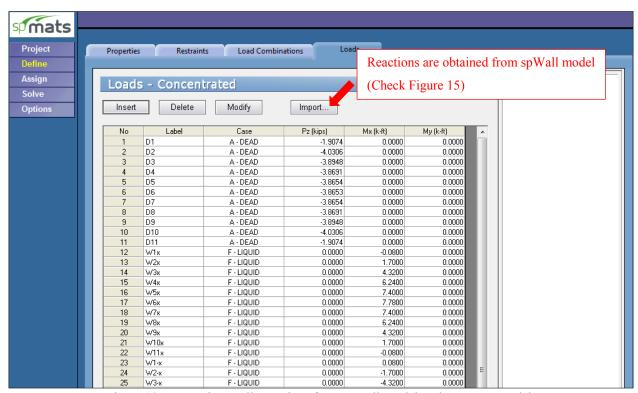
Figure 18 – Importing Wall Reactions from spWall Model to the spMats Model
