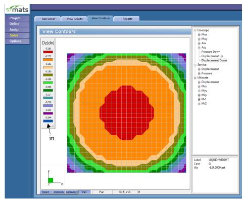
Figure 21 – Vertical (Down) Displacement Contour
