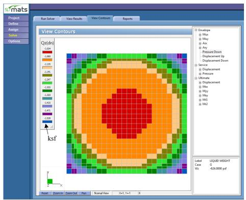
Figure 23 – Soil Pressure Envelope Contour
