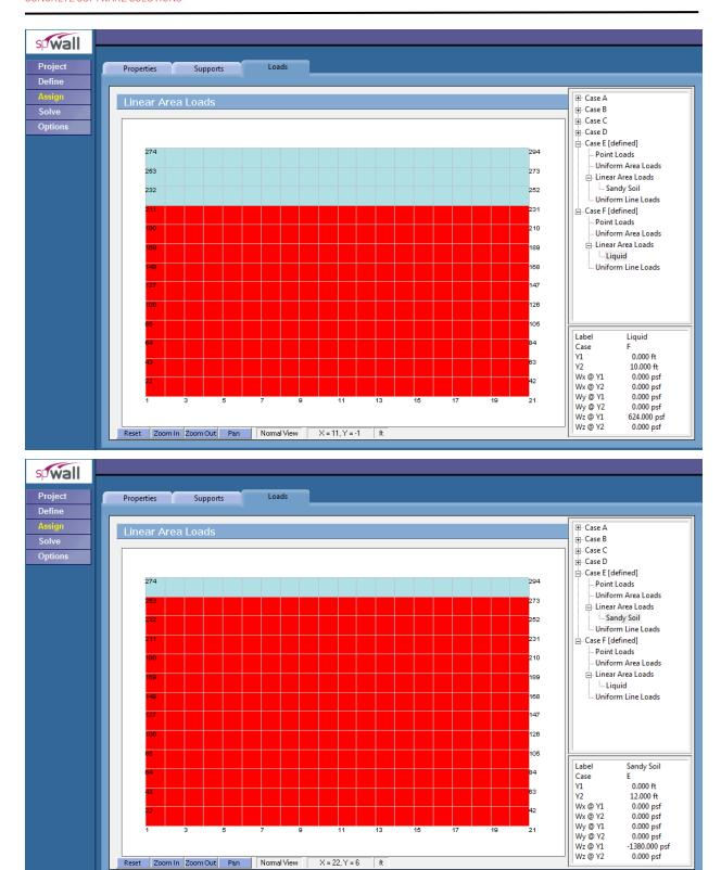
Figure 4 – Assigning Liquid and Soil Loads
