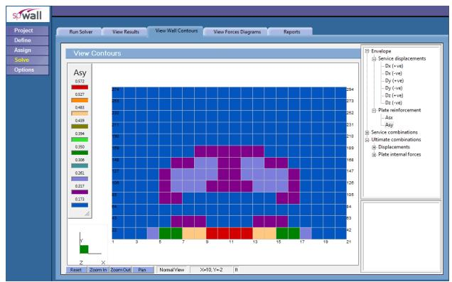
Figure 16 – Required Vertical Reinforcement
