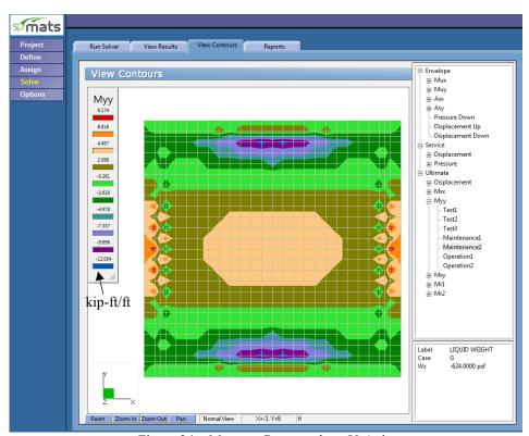
Figure 24 – Moment Contour along Y-Axis
