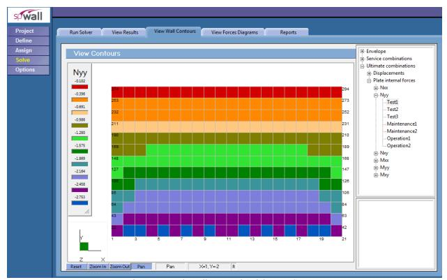
Figure 7 – Tank Wall Factored Axial Force Contour
