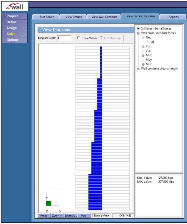
Figure 6 – Shear Wall Axial Load Diagram (spWall)
