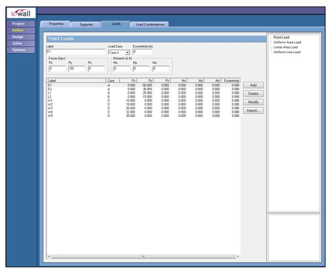
Figure 2 – Defining Loads for Shear Wall (spWall)
