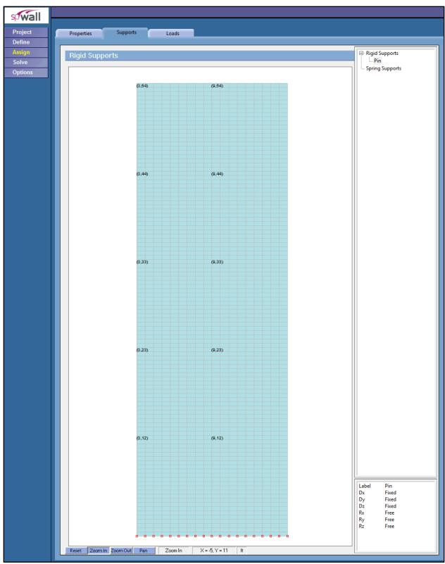
Figure 3 – Assigning Boundary Conditions for Shear Wall (spWall)
