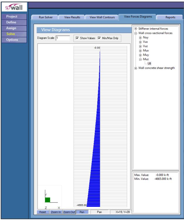
Figure 8 – Shear Wall Moment Diagram (spWall)
