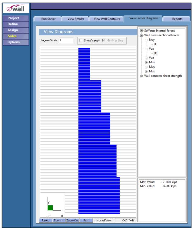
Figure 7 – In-plane Shear Diagram (spWall)
