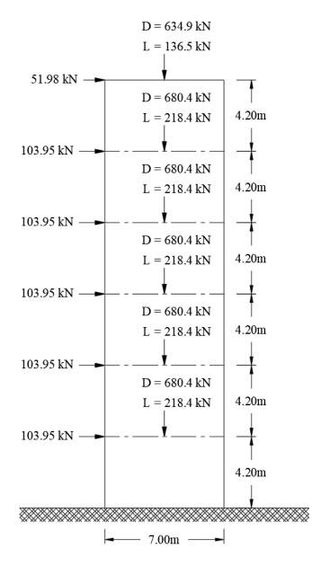
Figure 1 - Reinforced Concrete Shear Wall Geometry and Loading
