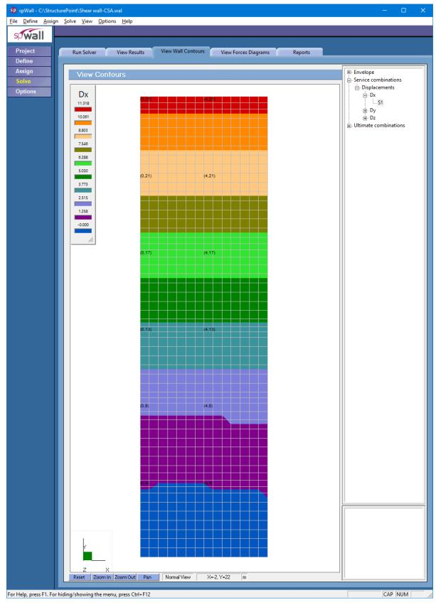
Figure 6 – Shear Wall Lateral Displacement Contour (spWall)
