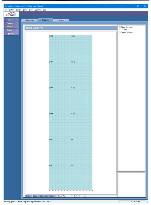
Figure 4 – Assigning Boundary Conditions for Shear Wall (spWall)
