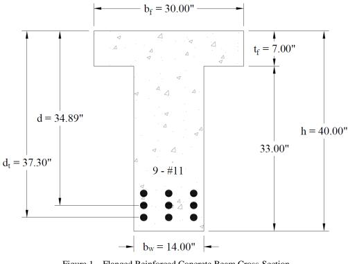
Figure 1 - Flanged Reinforced Concrete Beam Cross-Section
