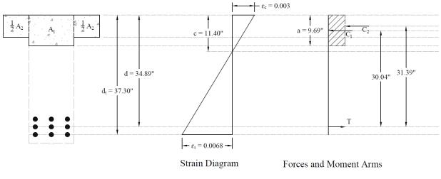
Figure 2 - Strain diagram and internal forces
