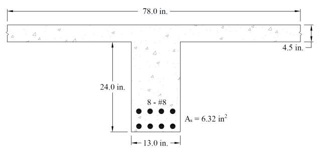
Figure 1 – Flanged Reinforced Concrete Beam (T-Beam) Cross-Section
