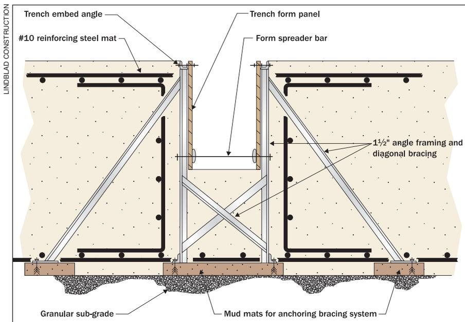
**Fig. 2. Trench Forming and Bracing System.** In order to avoid the possibility of “floating” the trench drain formwork, the bottom of the form was left open. By taking this precaution, Lindblad knew it would have to bush-hammer some of the bottom of the drain and establish proper pitch using overlay cements.
