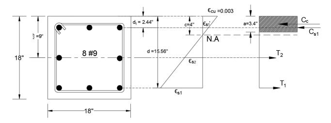
Use iterative procedure to determine  $\phi M_n$
