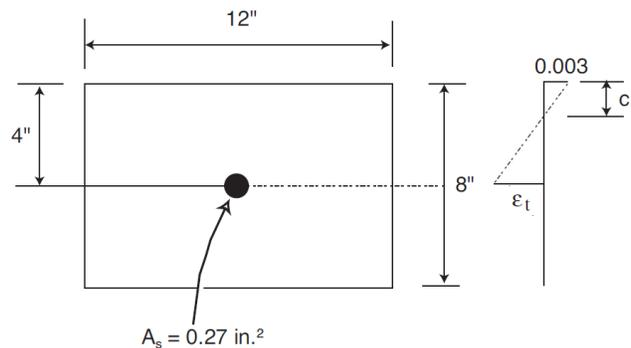
$$I_{cr} = 8.0 \times 0.34 \times (4 - 0.59)^2 + \frac{12 \times 0.59^3}{3} = 32.5 \text{ in.}^4 \quad \text{ACI 318-11 (Eq. 14-7)}$$
