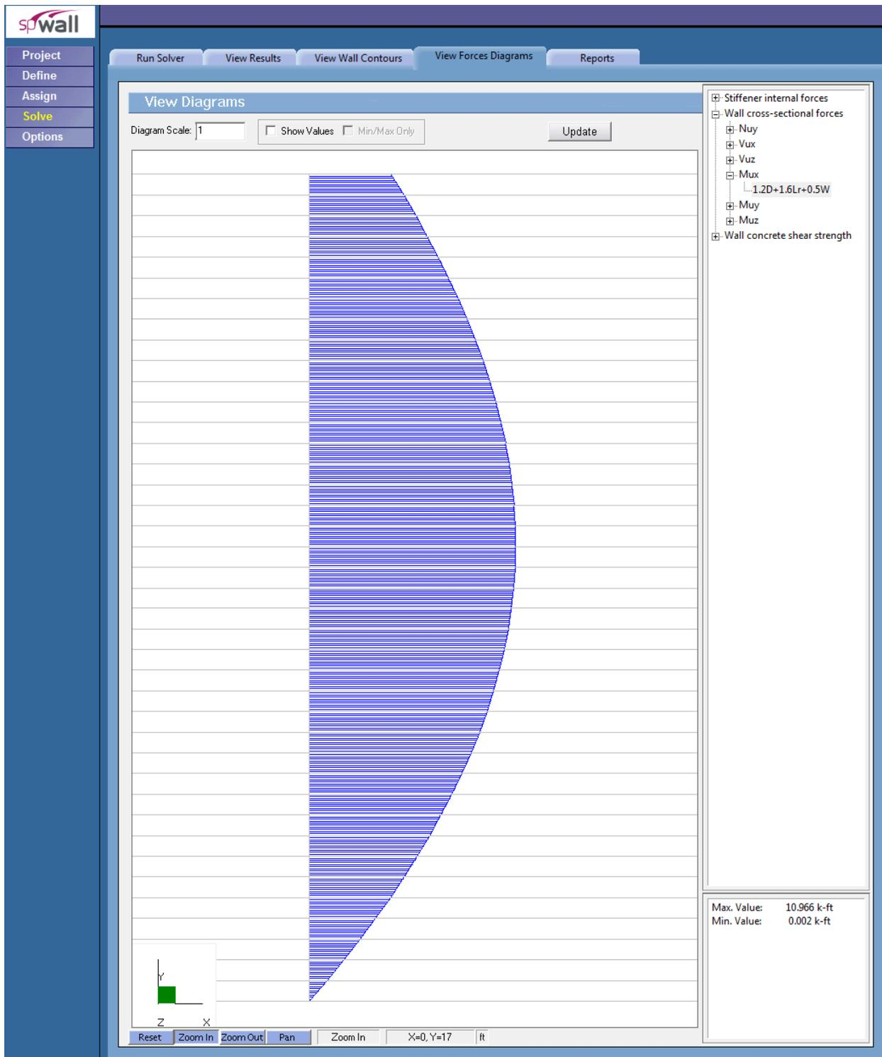
Figure 9 – Shear Wall Moment Diagram (spWall)
