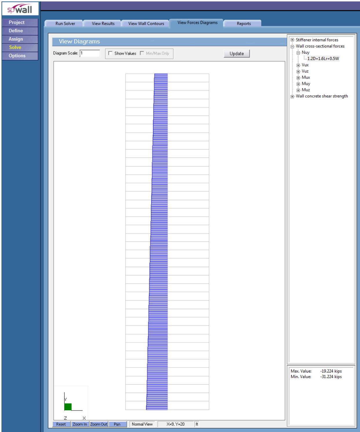
Figure 7 – Precast Wall Panel Axial Load Diagram (spWall)
