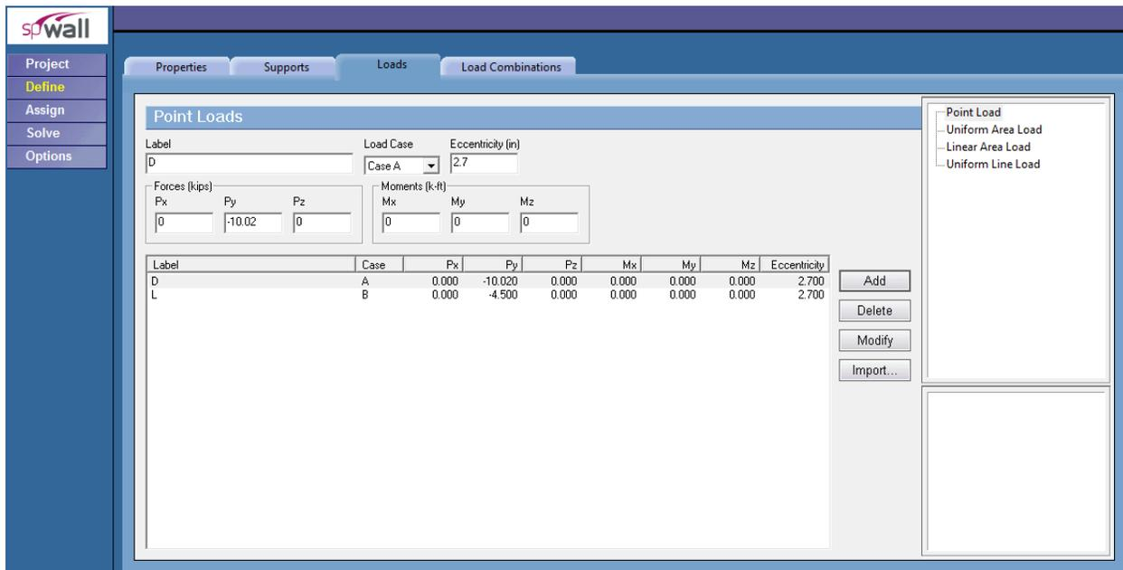
Figure 3 –Defining Loads for Precast Wall Panel ([spWall](#))
