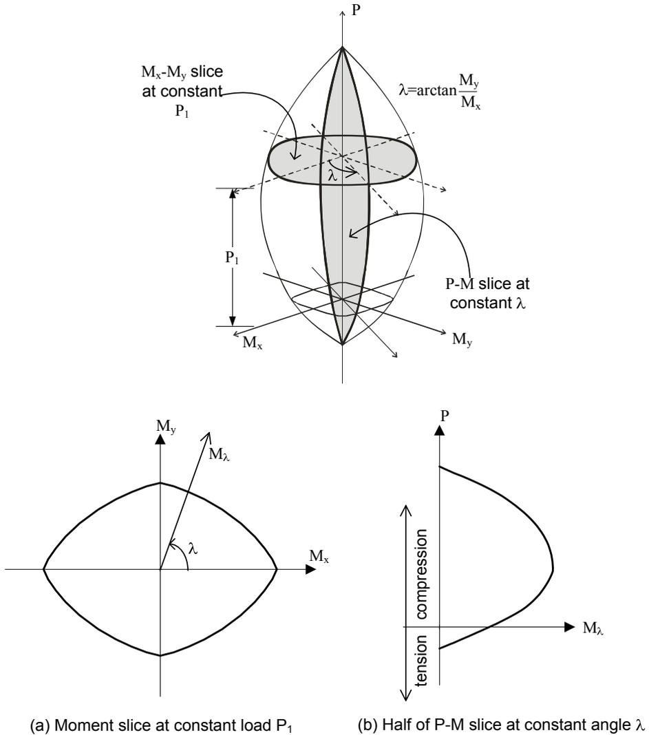
Figure 2-6 Interaction Surface for Combined Axial Load and Biaxial Bending
