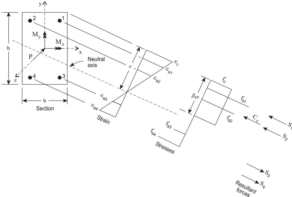
Figure 2-1 Analysis of Reinforced Section
