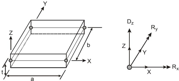
Figure 2-4 The Plate Finite Element
