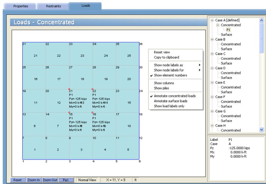
Alternatively, you can click on the **Assign** button located on the toolbar, and then on the LOADS tab. If columns or piles have been assigned to the model, they are displayed in the color specified for COLUMN or PILES in the DISPLAY SETTINGS. If it is preferred not to show columns or piles, right-click on empty space on the view window, and then uncheck Show Columns or Show Piles on the pop-up menu.
