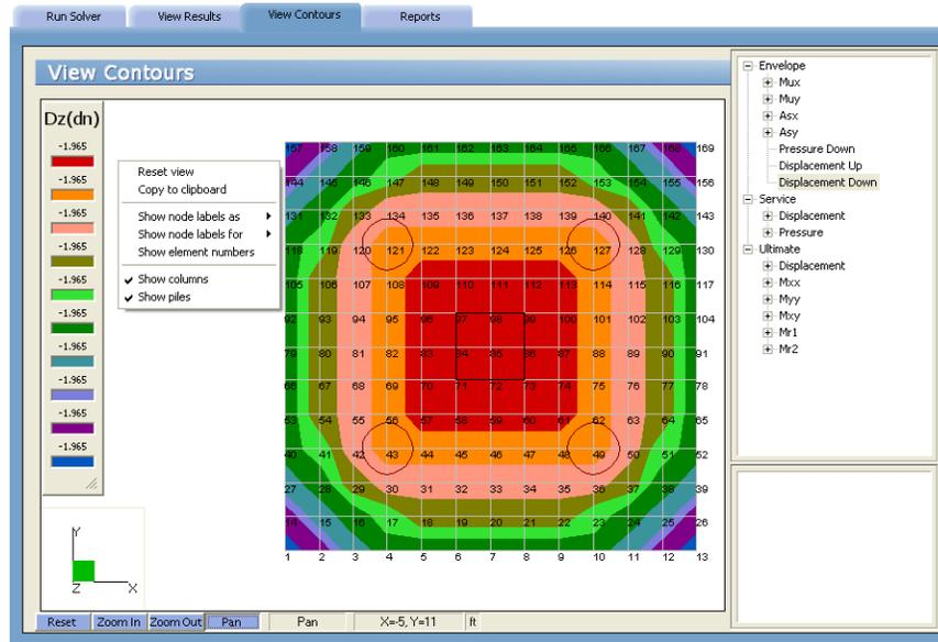
If columns have been assigned to the model, they are displayed to scale in black color. If piles have been assigned to the model, they are displayed to scale in dark red color. To not show columns or piles, right-click on empty space on the view window, and then uncheck Show Columns or Show Piles on the pop-up menu.
