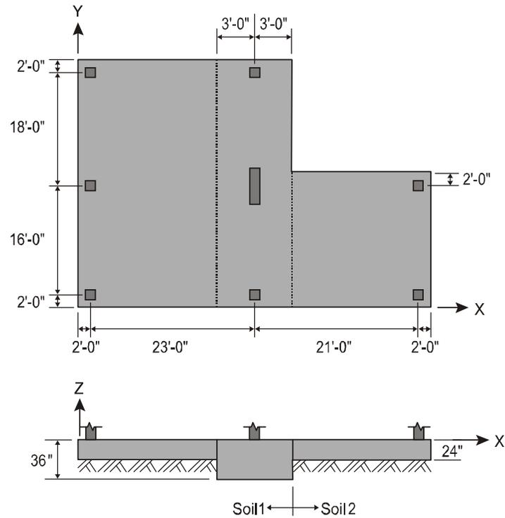
The mat is supported on two types of soil, Soil-1 and Soil-2, as shown in the figure. Use the following data:
