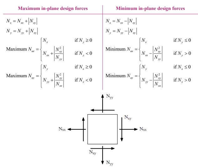
In the above equations,  $N_{xx}$ ,  $N_{yy}$  and  $N_{xy}$  correspond to the element internal in-plane forces at the element center.
