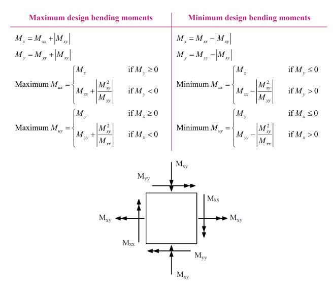
In the above equations,  $M_{xx}$  and  $M_{yy}$  correspond to the element internal bending moments at the element center, while  $M_{xy}$  corresponds to the element internal torsional moment at the element center.
