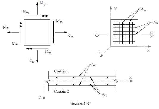
Figure 2.11 – Design Forces and Location of Bars
