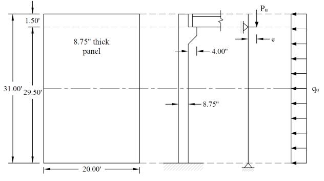
Figure 8.1 – Concrete Wall Geometry
