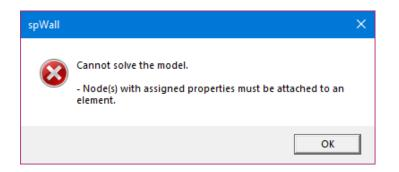
The Program also ensures that null stiffener elements exist within a plate element. If a null stiffener is placed outside the plate element, the following Error message is displayed.
