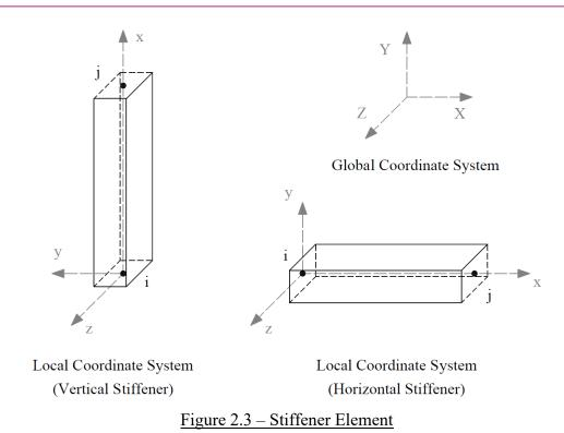
The properties of the stiffener section, area (A), Inertia  $(I_y, I_z)$  and torsional constant (J) are calculated as follows
