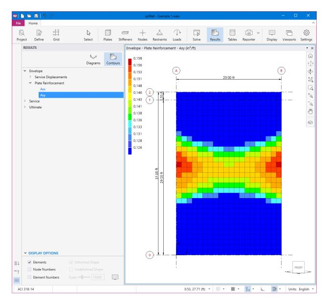
Please be advised that spWall displays the total flexure reinforcement, for each element, for two curtains of reinforcement.
