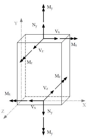
Figure 2.9 – Wall Cross-sectional Forces
