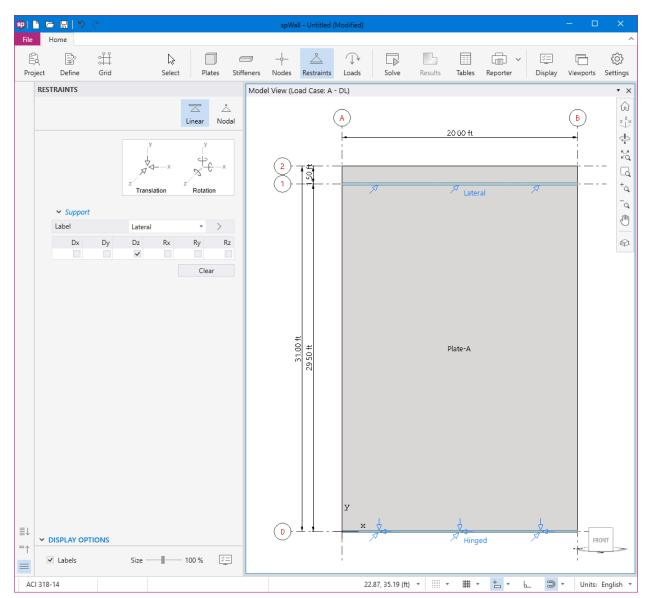
• Apply LATERAL support to the top null stiffener as shown in the figure below.
