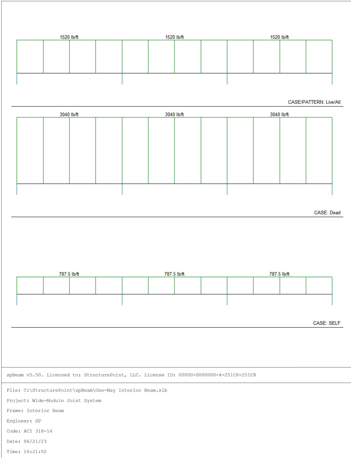
Figure 28 – spBeam Model – Loads (Including Live Load Patterning)
