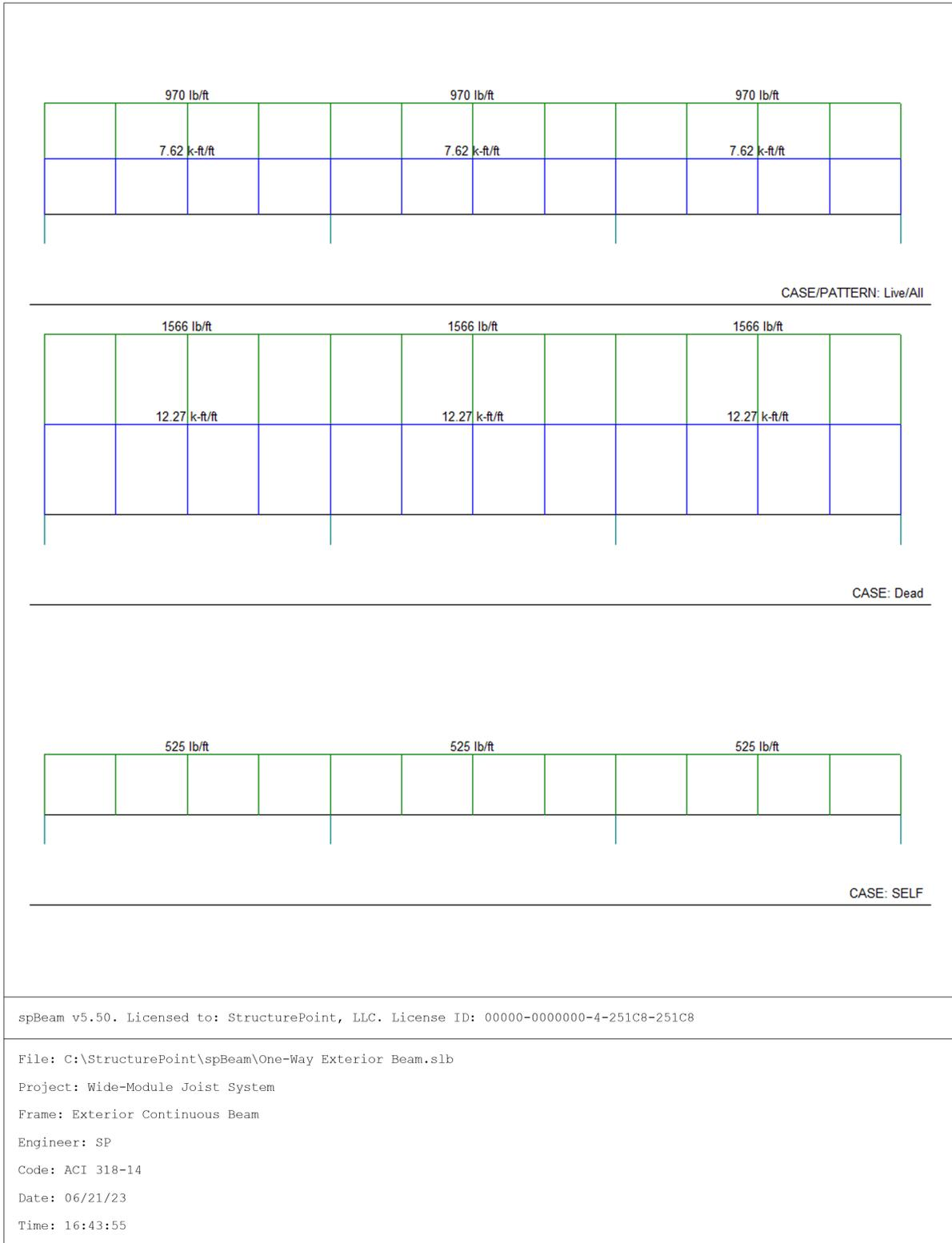
**Figure 39 – spBeam Model – Loads (Including Live Load Patterning)**
