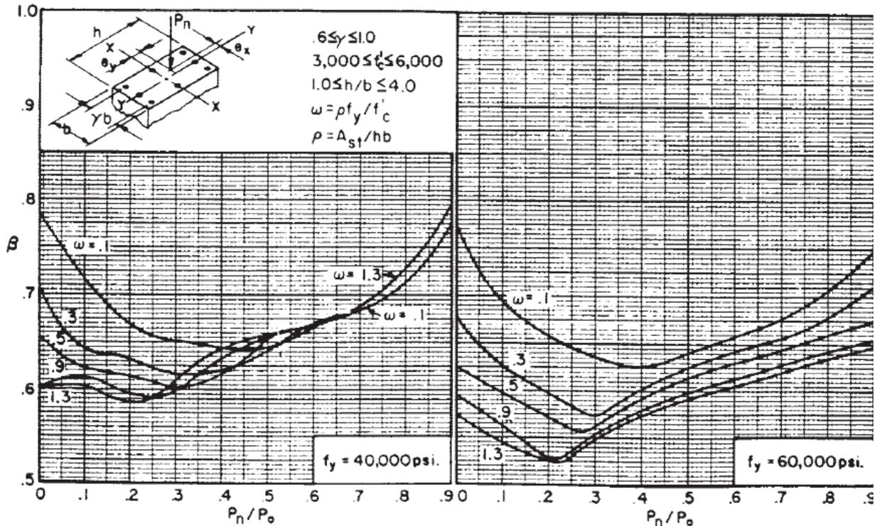
Figure 5 – Sample of Figure 7-15 (Biaxial Design Constants - 4 Bar Arrangement)
