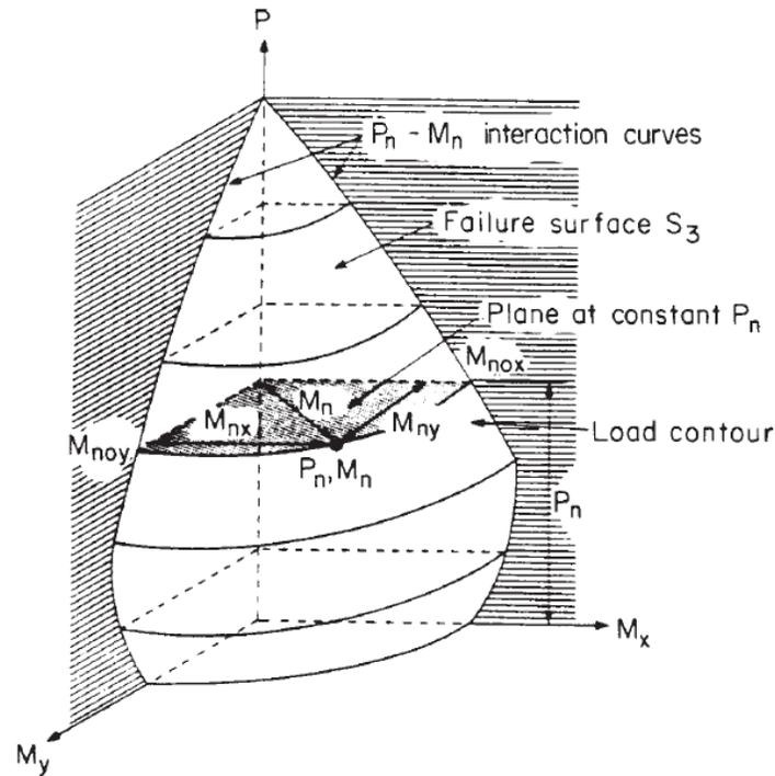
Figure 10 – Bresler Load Contours for Constant  $P_n$  on Failure Surface  $S_3$
