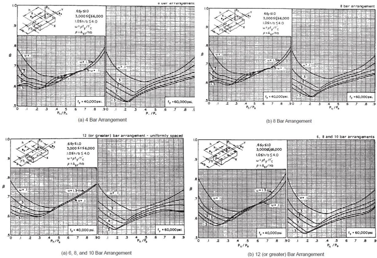
Figure 16 – Biaxial Design Constants
