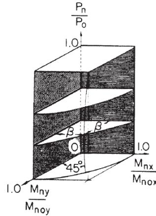
Figure 14 – Nondimensional Load Contour at Constant  $P_n$
