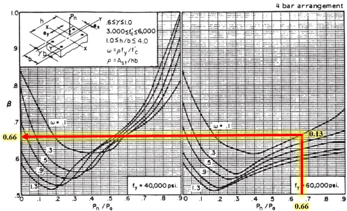
Figure 18 – Biaxial Design Constants (4 Bar Arrangement)
