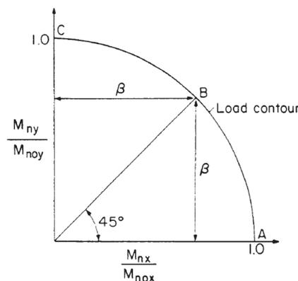
Figure 13 – Nondimensional Load Contour at Constant  $P_n$
