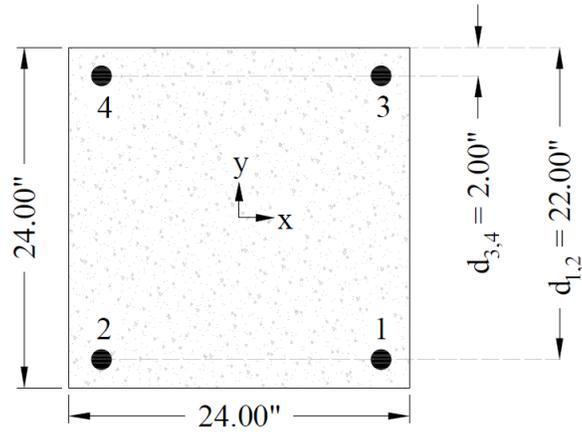
Figure 2 – Reinforced Concrete Column Cross-Section and Reinforcement Locations
