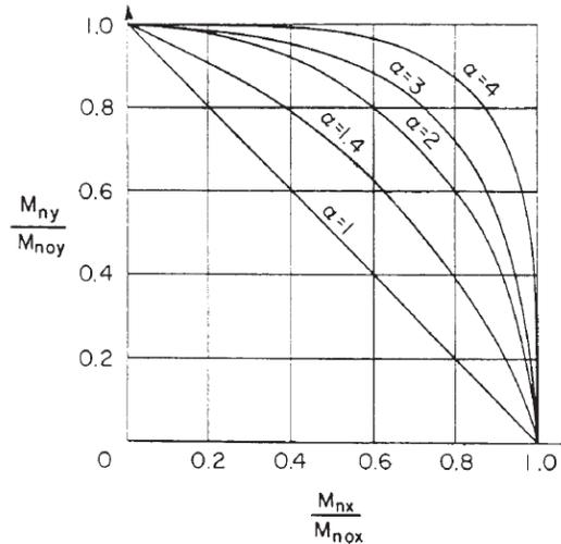
**Figure 11 – Interaction Curves for Bresler Load Contour Method**
