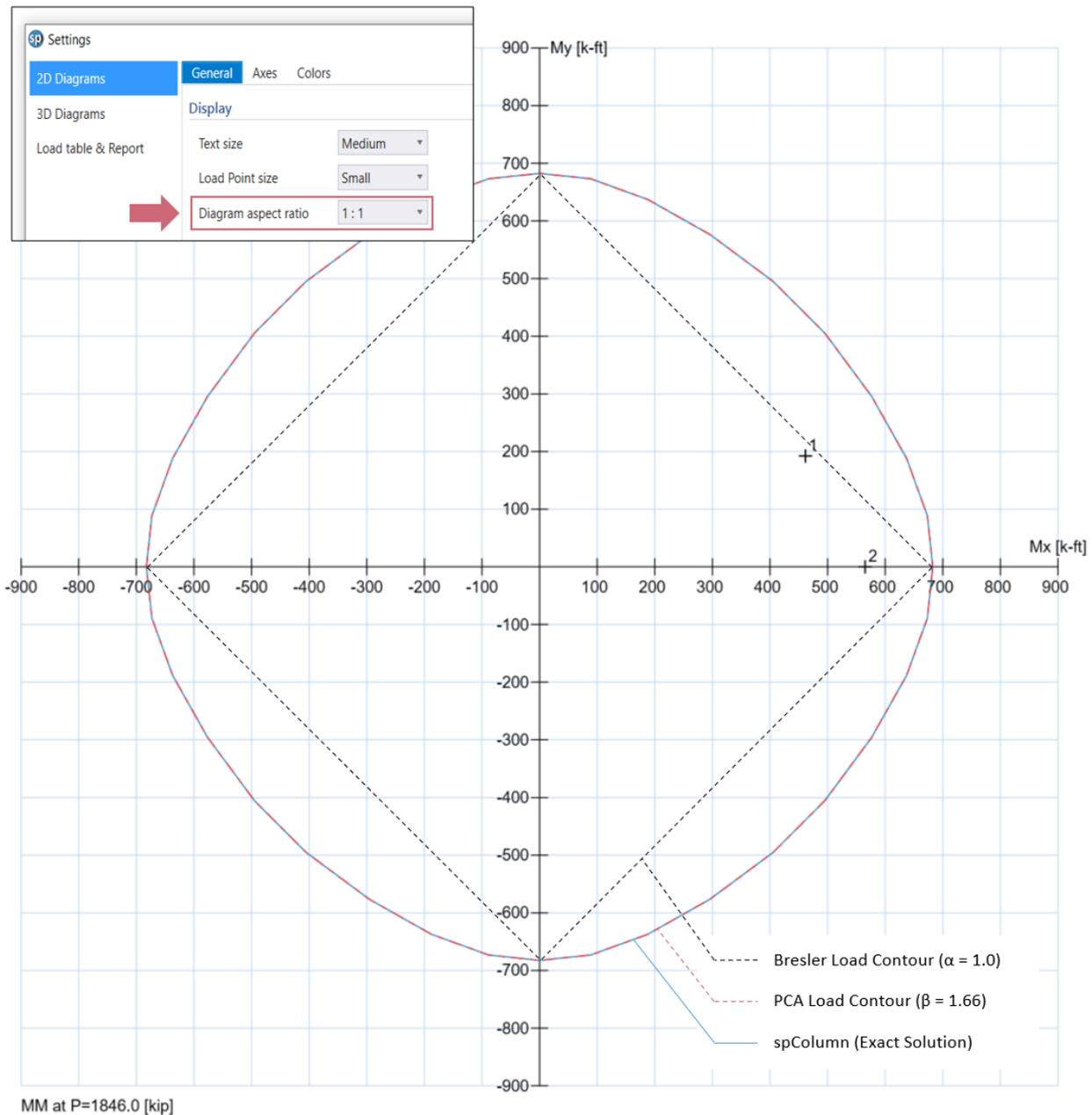
Figure 23 – Column Section  $M_{nx}$ - $M_{ny}$  Contour at  $P_n = 1846$  kip (spColumn 2D/3D Viewer)
