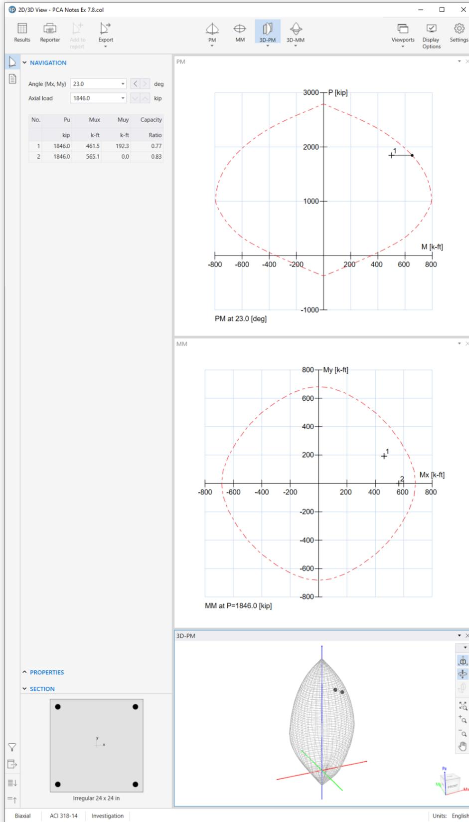
Figure 25 – 2D/3D Biaxial Interaction Diagram Viewer (spColumn)
