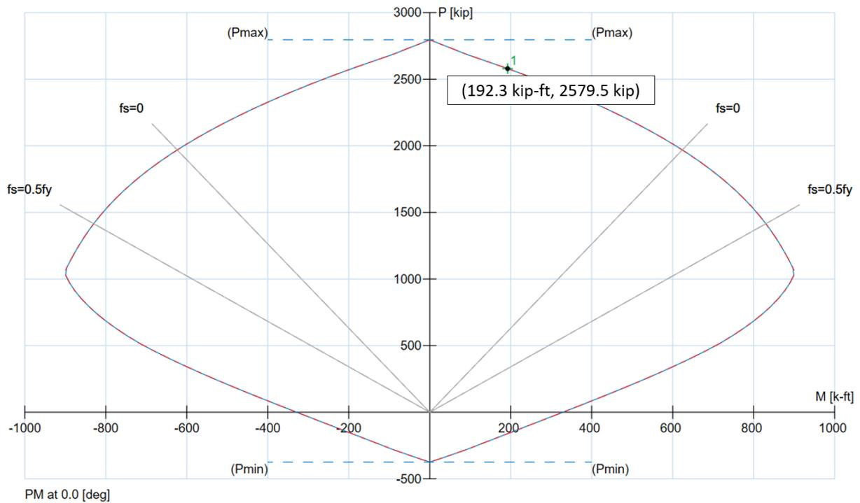
**Figure 9 – Column Uniaxial Interaction Diagram ( $P_{noy}$  and  $M_{ny\_req}$ )**
