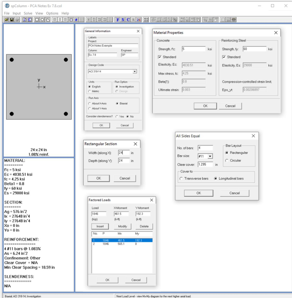
Figure 20 – Generating spColumn Model
