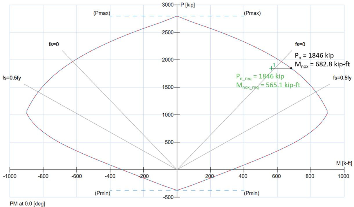
Figure 6 – Column Section Capacity Interaction Diagram (spColumn)
