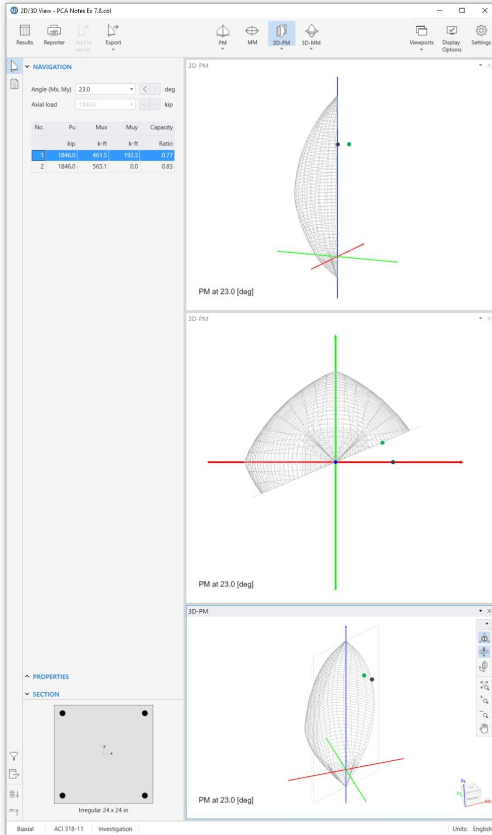
Figure 27 – 3D Visualization of Failure Surface with a Vertical Plane Cut at 23° (spColumn)
