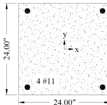
Figure 1 – Reinforced Concrete Column Cross-Section
