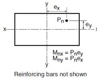
Figure 3 – Notation for Biaxial Loading
