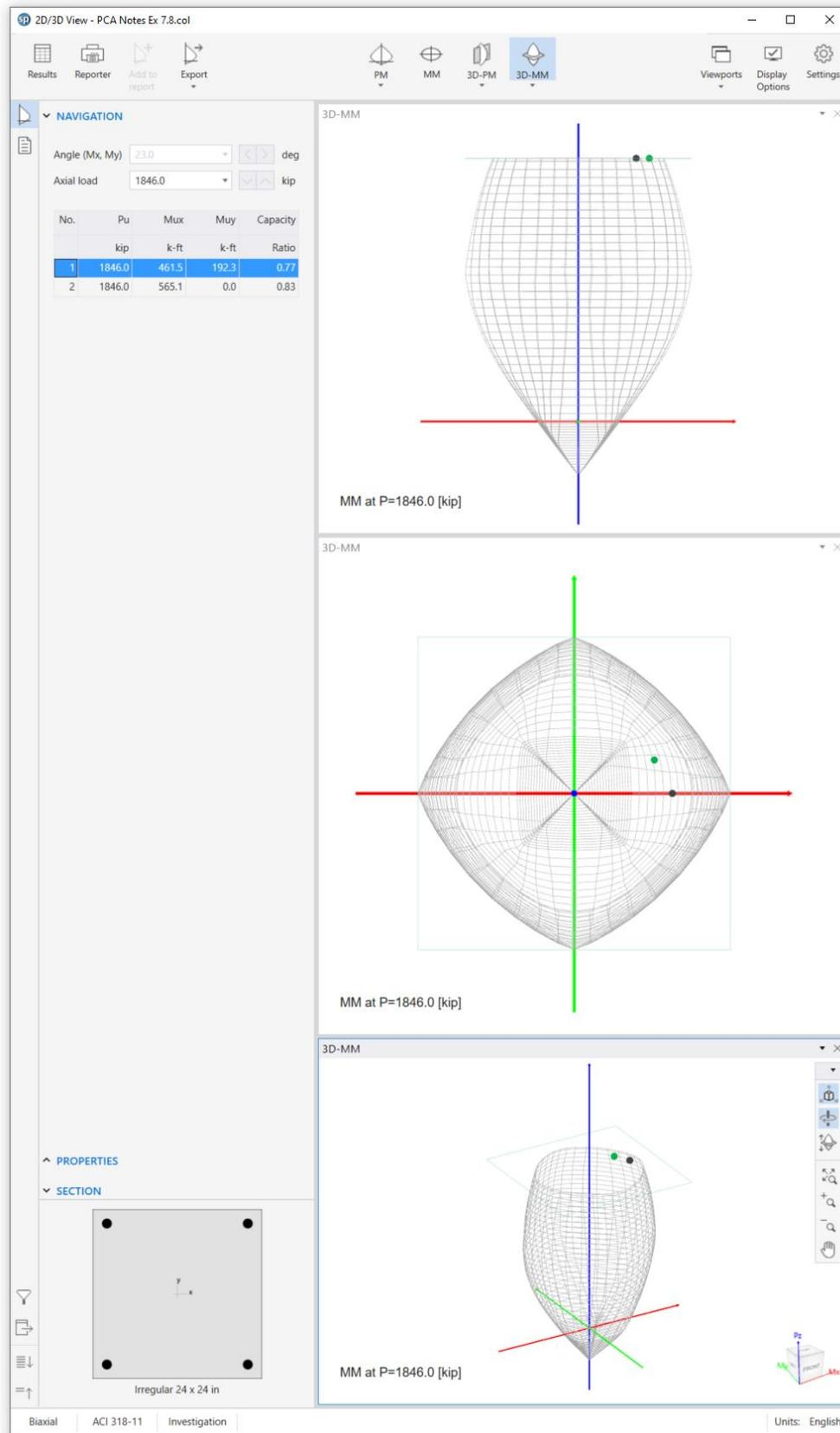
Figure 26 – 3D Visualization of Failure Surface with a Horizontal Plane Cut at P = 1846.0 kip (spColumn)
