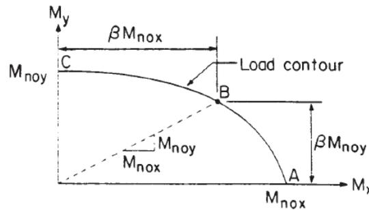
Figure 12 – Load Contour of Failure Surface  $S_3$  along Plane of Constant  $P_n$
