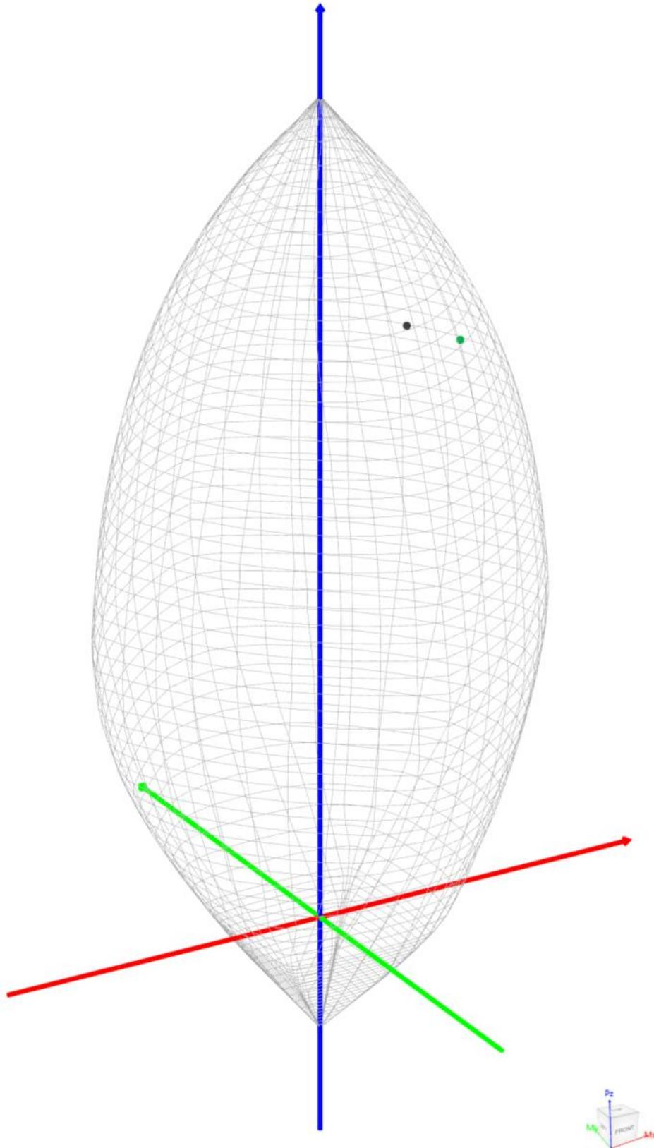
Figure 24 – Interaction Diagram in Two Directions (Biaxial) (spColumn)
