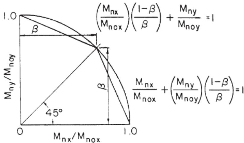
Figure 17 – Bilinear Approximation of Nondimensionalized Load Contour
