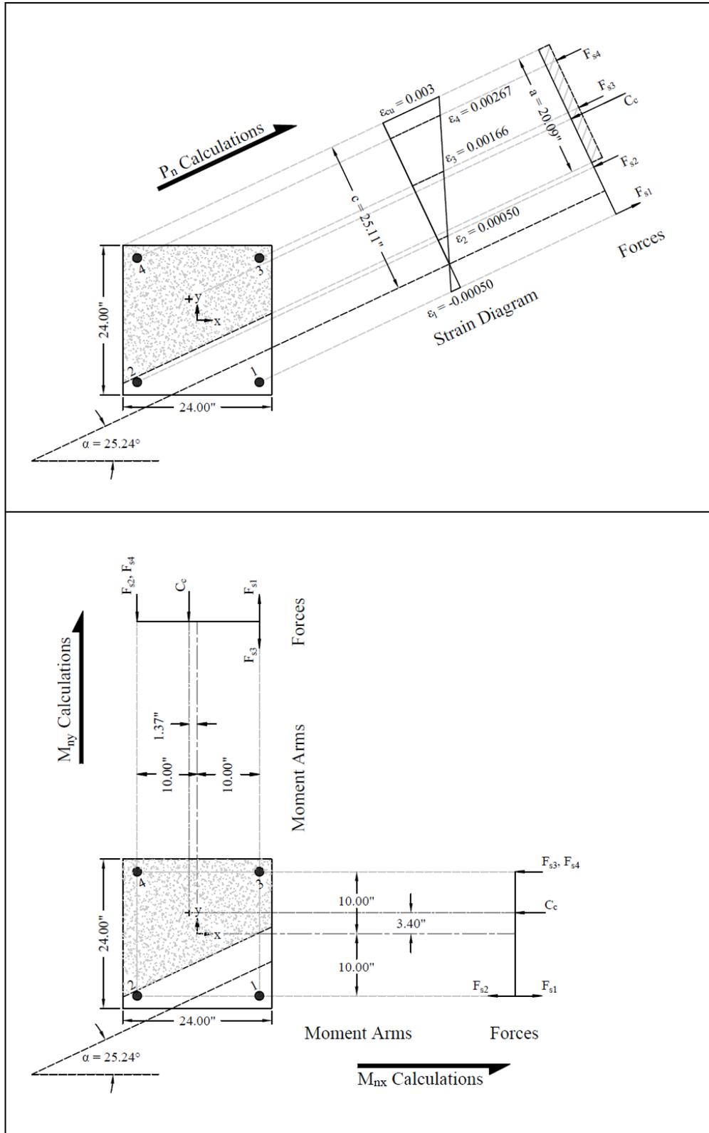
Figure 19 – Column Biaxial Bending – Axial Interaction Exact Method.
