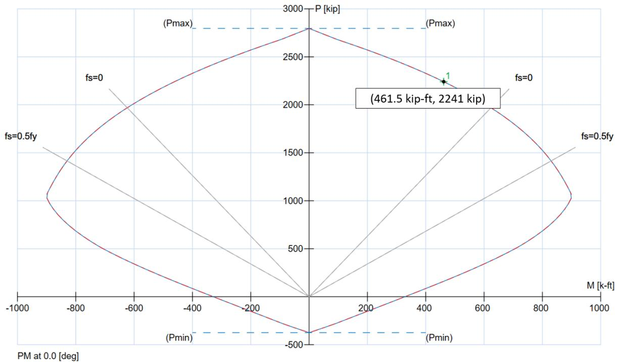
**Figure 8 – Column Uniaxial Interaction Diagram ( $P_{nox}$  and  $M_{nx\_req}$ )**
