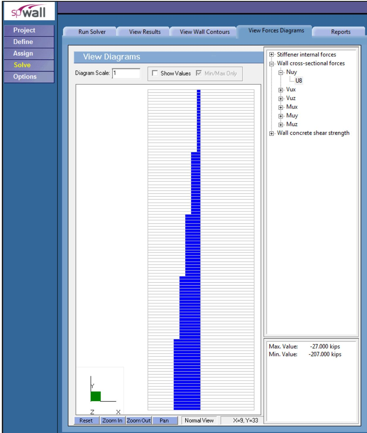
Figure 6 – Shear Wall Axial Load Diagram (spWall)
