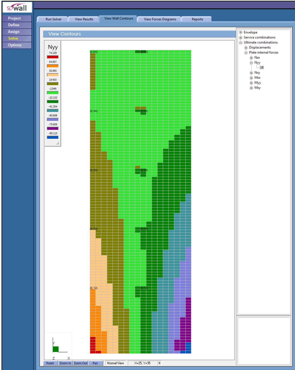
Figure 4 –Factored Axial Forces Contour Normal to Shear Wall Cross-Section (spWall)
