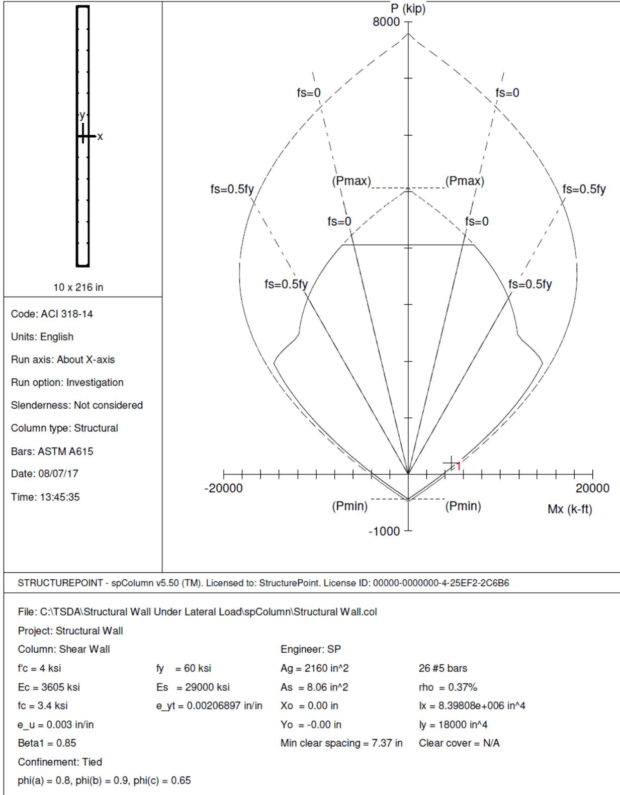
**Figure 11 – Shear Wall Interaction Diagram (X-Axis, In-Plane) (spColumn)**
