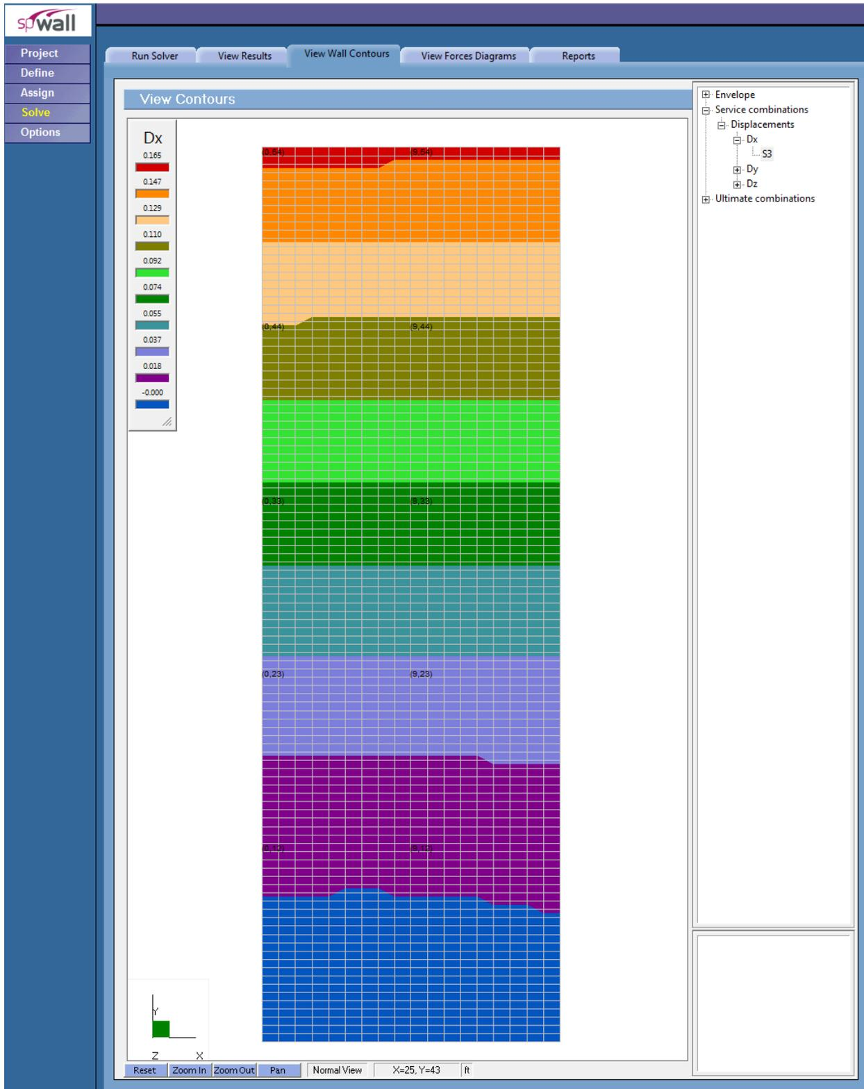
Figure 5 – Shear Wall Lateral Displacement Contour (spWall)
