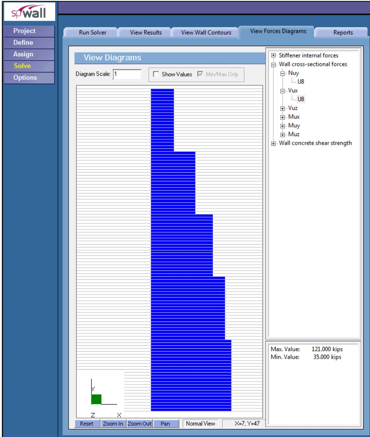
Figure 7 – In-plane Shear Diagram (spWall)
