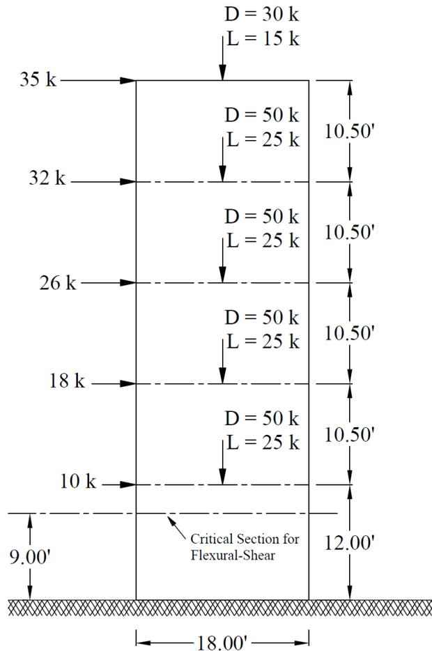
**Figure 1 – Reinforced Concrete Shear Wall Geometry and Loading**
