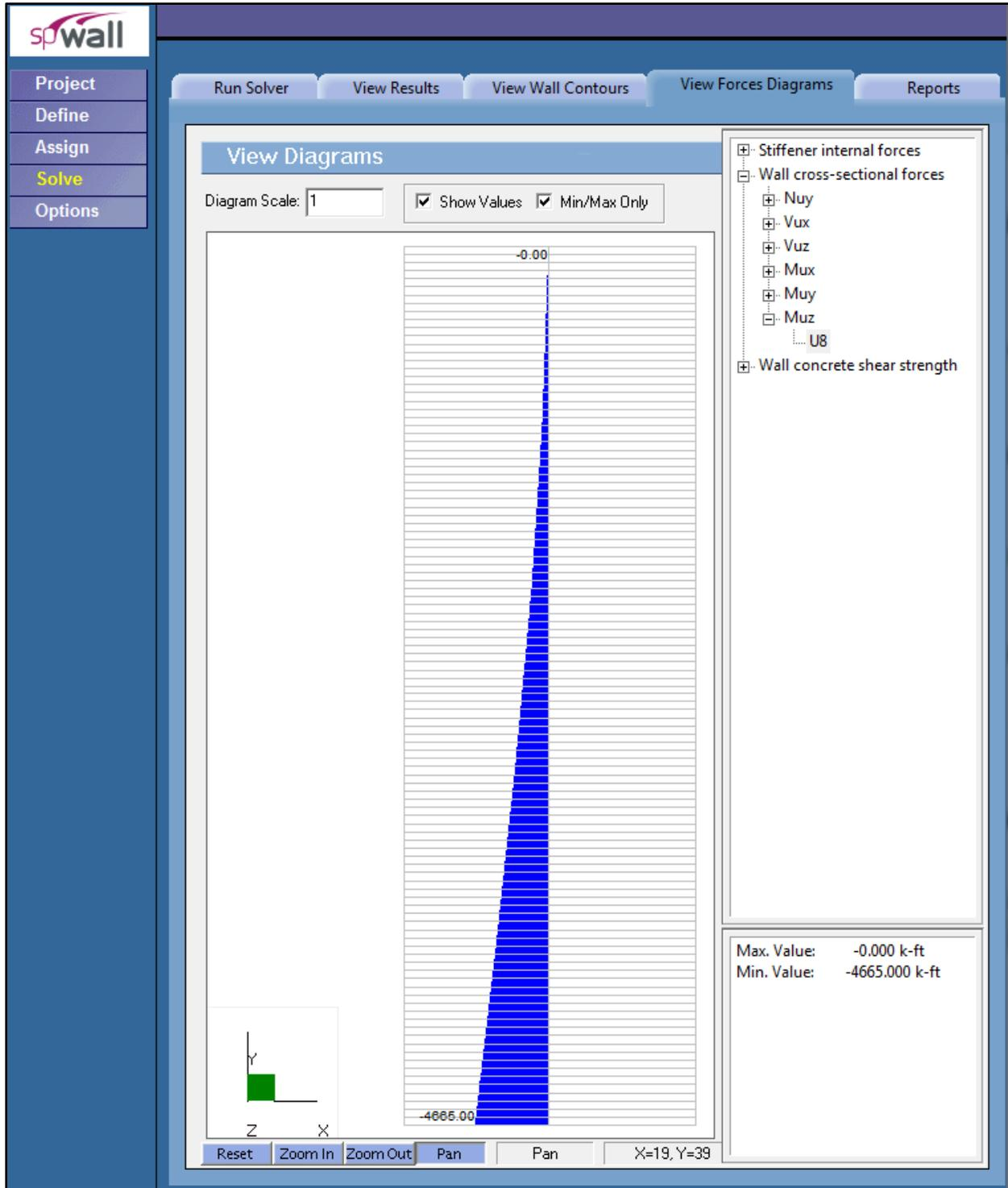
Figure 8 – Shear Wall Moment Diagram (spWall)
