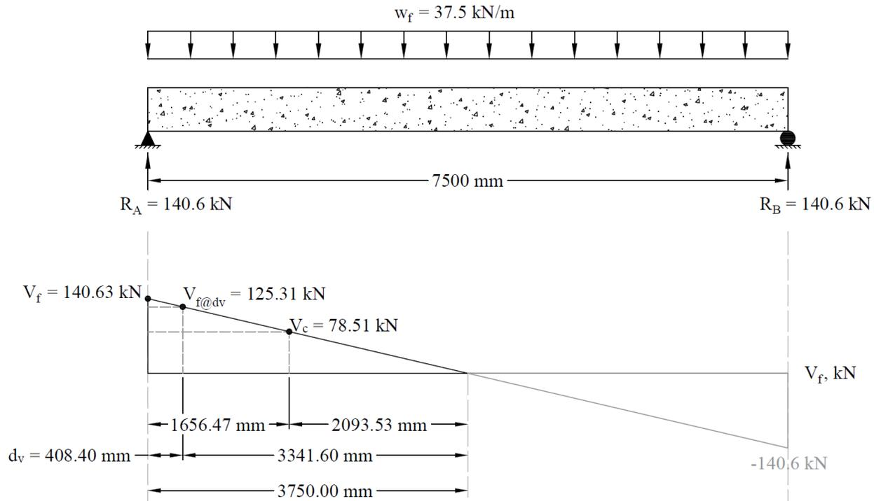
**Figure 4 – Shear Diagram for Simply Supported Beam**
