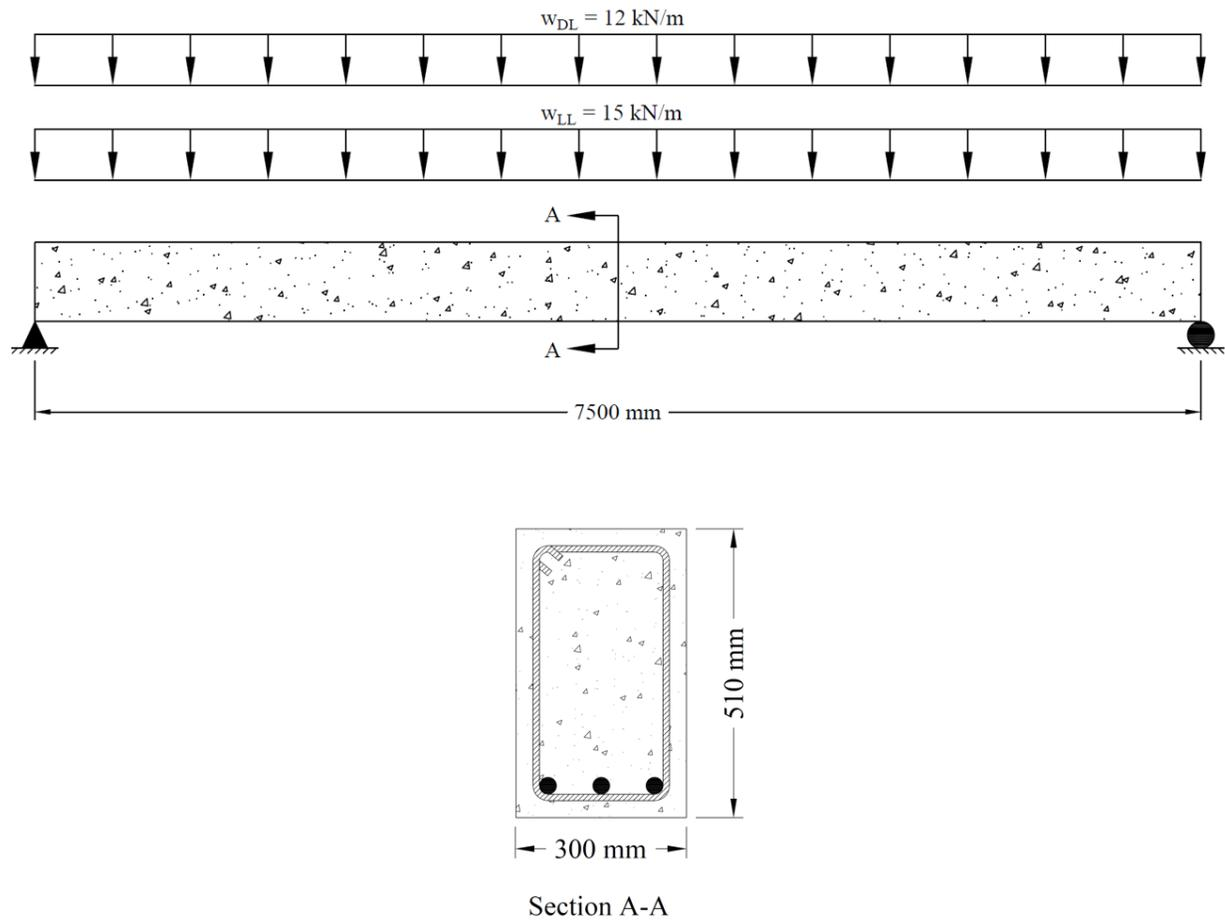
Figure 1 – Rectangular Simply Supported Reinforced Concrete Beam
