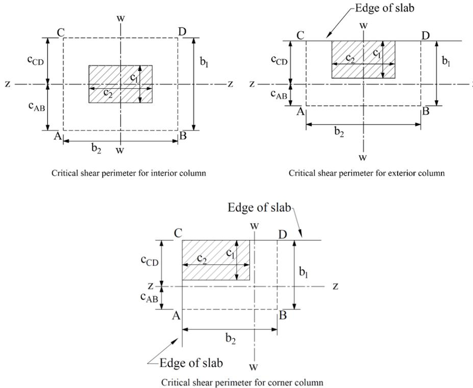
**Figure 5 – Critical Shear Perimeters for Columns**
