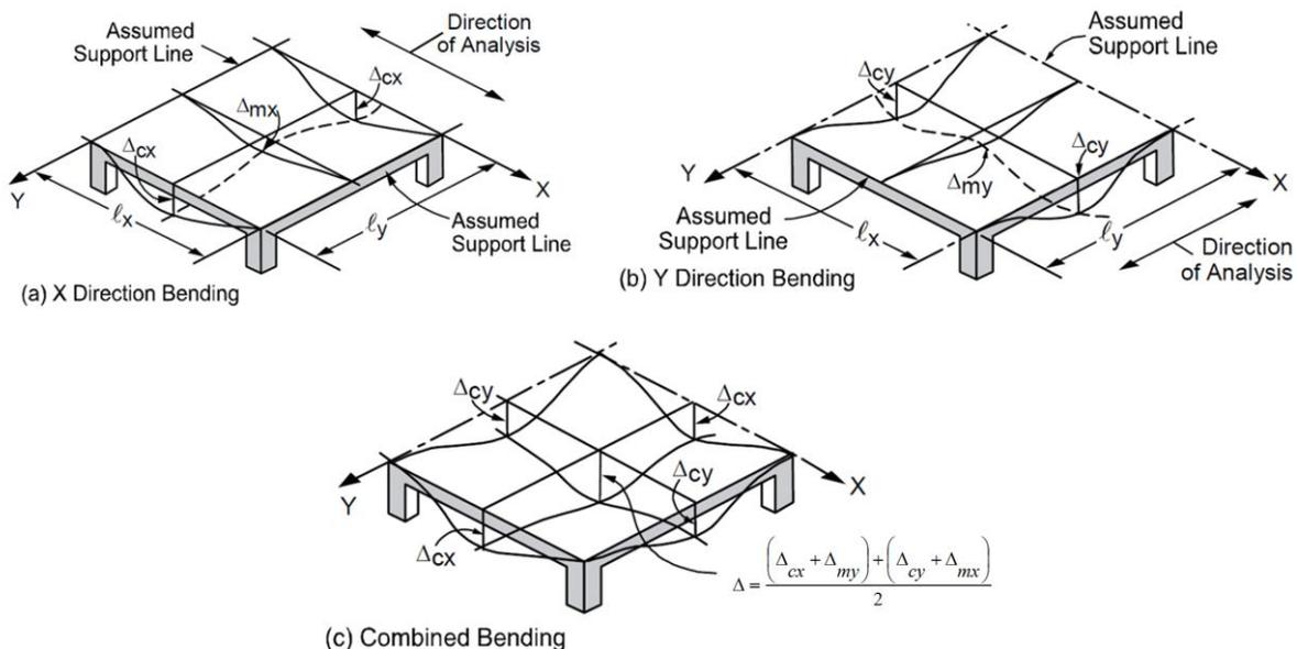
Figure 14 – Deflection Computation for a rectangular Panel
