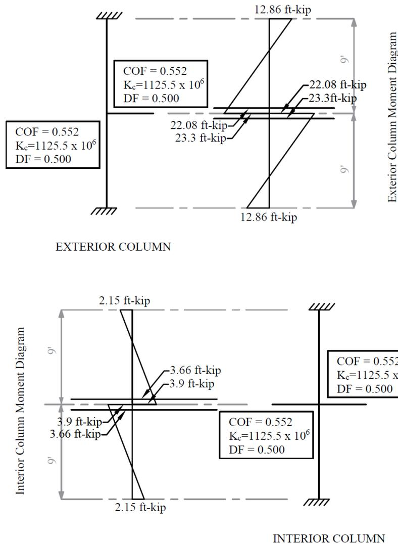
Figure 10a - Column Moments (Unbalanced Moments from Slab-Beam)
