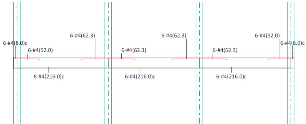
Middle Strip Flexural Reinforcement
