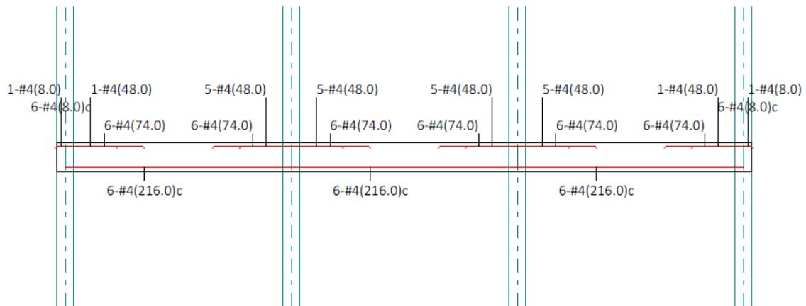
Column Strip Flexural Reinforcement
