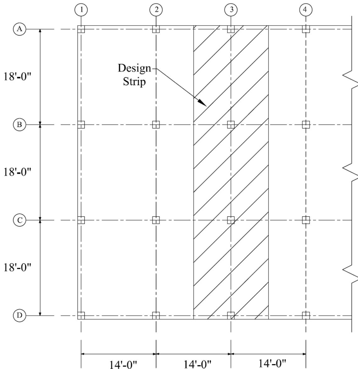
Figure 1 - Two-Way Flat Concrete Floor System
