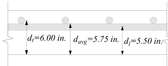
Figure 2 - Two-Way Flat Concrete Floor System
