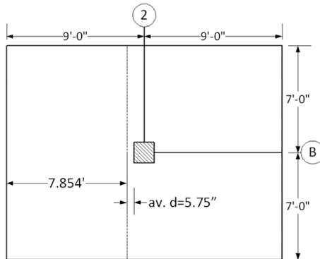
Figure 3 – Critical Section for One-Way
