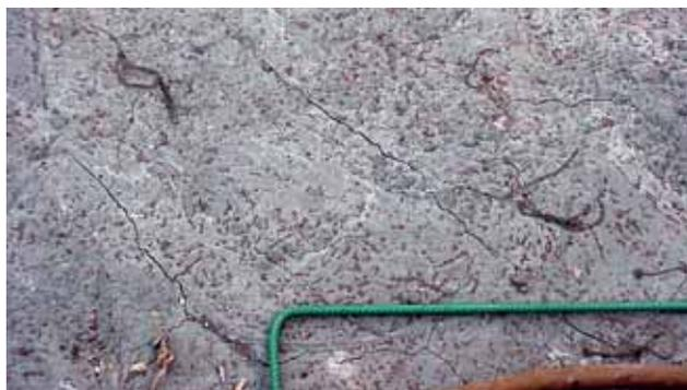
A concrete core removed from a column foundation shows the extent of thermal cracking.
