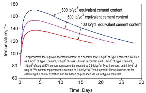
Mix designs for a 10-foot-thick slab evaluated by modeling of temperatures.
